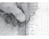
Step 3.5. Use a glove or other protective cloth to pull off the loosened jacket slug. **Do not touch** the hot jacket slug with bare fingers. The slug will be very hot and will burn!
