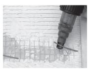
Step 4.4. With either type of jacket, if the jacket slug doesn't easily pull off you may need to use your heat gun to gently warm the slug, which should soften and loosen it for you. Use the heat gun (set to about 500°F) and move the gun back and forth under the jacket slug for about 3 or 4 seconds, or until it can be easily removed.
