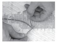
Step 4.8. Use the small screwdriver, paper clip, fingernail, or similar instrument to pry between the braid and make an opening through which to pull the heating wires. Pull each wire through the braid.
