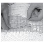
Step 4.9. Pull the braid straight out to make it into a pigtail.
