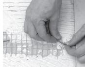
Step 4.3. Gently bend the cable at the score to break through the jacket all the way around the cable, then pull off the slug
