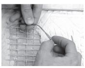
**Step 3.6.** Loosen the braid by pushing back on the braid about 1/2" and cause the ends of the heating wires to be exposed.
