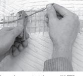
Some of our products have an "XLPE" jacket that is a somewhat hard material that can be lightly "scored" with a scoring tool or sharp blade. Use the scoring tool to carefully score the jacket about 2.5" from the end of each lead. Do this by placing the cable lead into the V-notch of the tool and rotating the tool only one or two revolutions around the cable. Do not place any additional pressure on the tool head to cut deeper. Let the tool apply its own spring-loaded pressure.
