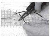
Step 4.13. Use the 16 AWG setting on the wire strippers to strip off exactly 1/2' of the insulation from both ends of the jumper wires.
