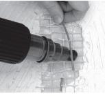
Step 3.4. With either type of jacket, if it doesn't easily pull off you may need to use your heat gun to gently warm the slug, which should soften and loosen it for you. Use the heat gun (set to about 500°F) and move the gun back and forth under the jacket slug for about 3 or 4 seconds, or until it can be easily removed.
