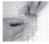
Step 3.8. Use the small screwdriver, paper clip, fingernail, or similar blunt instrument to pry between the braid and make an opening through which to pull the heating wires. Pull each wire through the braid.
